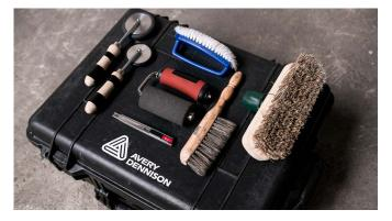
To ensure the best end-results, we advise to prepare prior the application the availability of a suitable brush for cleaning the wall and a set of application rollers depending on the texture and size of corrugations of the work surface.
