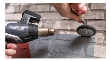
> As a final step, repeat the re-heating and roller step on the outer lining of the graphic once again. This is to ensure that the edges are properly sealed and to avoid any unwanted delamination in time. In case of multi panel application it is recommended to apply an overlap of at last 13 mm.
