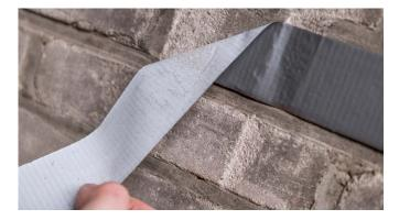
> Prior to starting the application, we advise to test on a small surface the anchorage of the substrate on the surface. This will also indicate whether proper level of cleanliness has been achieved to get sufficient anchorage.
